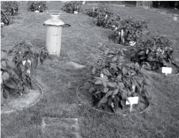
Figure 1: Irrigation experiment on simple drainage lysimeters at Karcag
