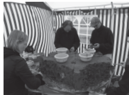
Figure 5: Sampling of a freshly cut soil slice
