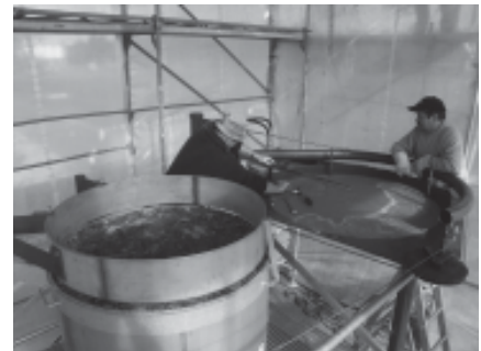
Figure 4: Preparation for the first cut of a soil slice
