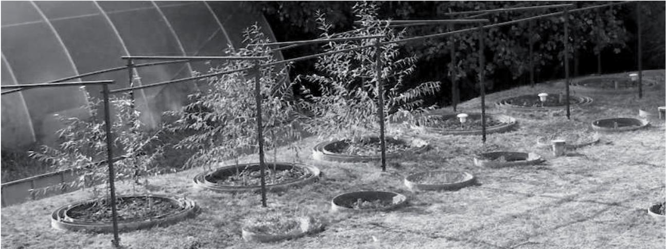
Figure 1: Energy willows in the weighable lysimeters at Karcag
