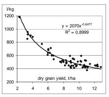
Figure 2: Relationship between the maize grain yield and the specific water consumption
