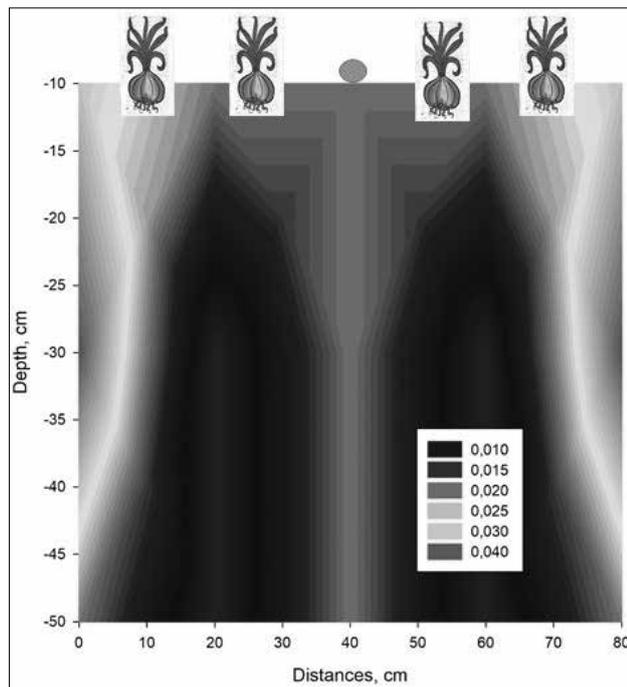
Figure 5. Soil EC in KSC treatment 2 after irrigation in April in dS/m.
