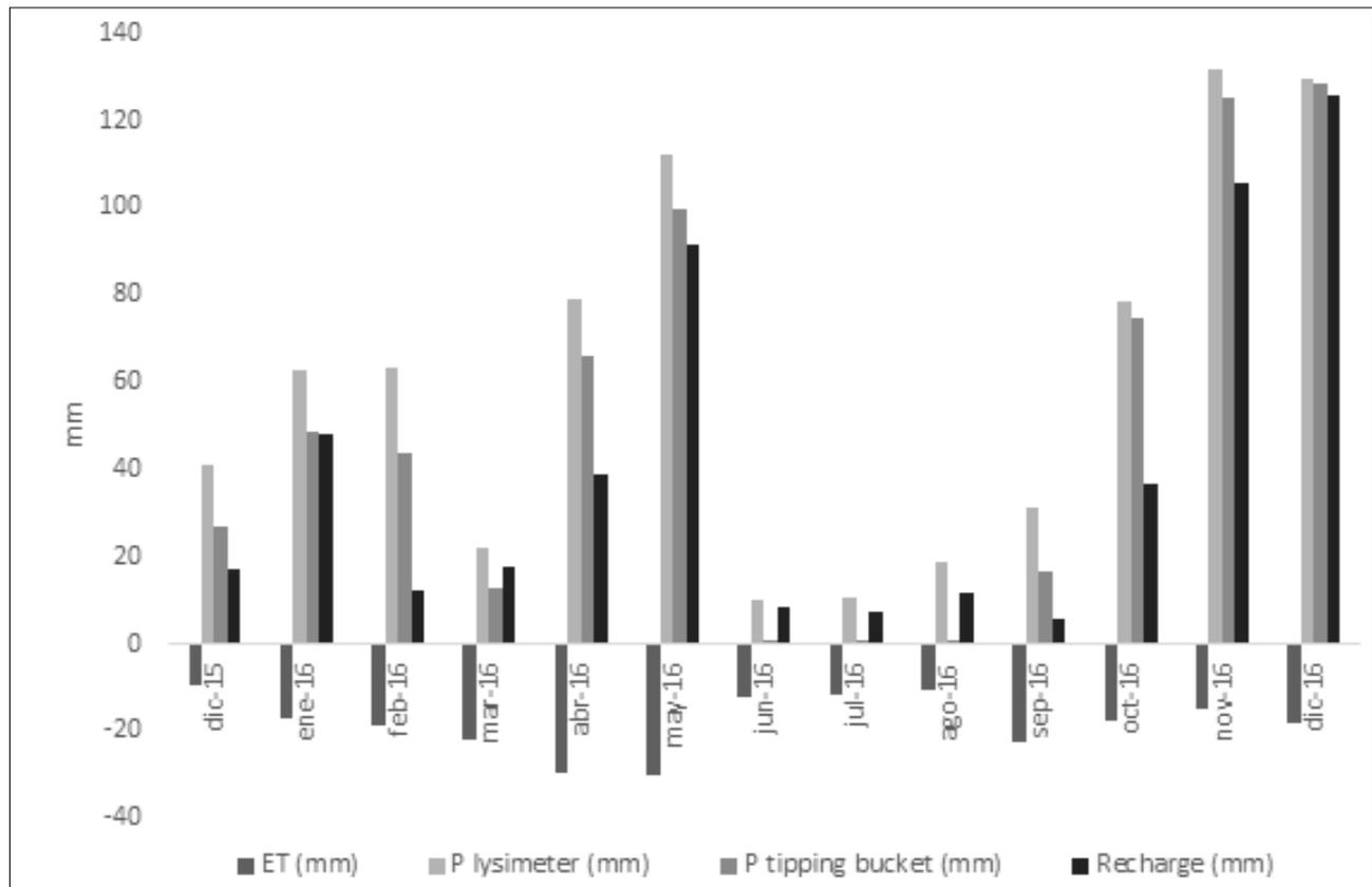
Figure 4: Monthly evapotranspiration (ET) and rainfall (P), both calculated using lysimeter data, rainfall measured with the tipping bucket rain gage (P<sub>t</sub>), and recharge (R), measured as weight increase due to drained water of the lysimeter into the sample vessel, from December 2015 to December 2016.
