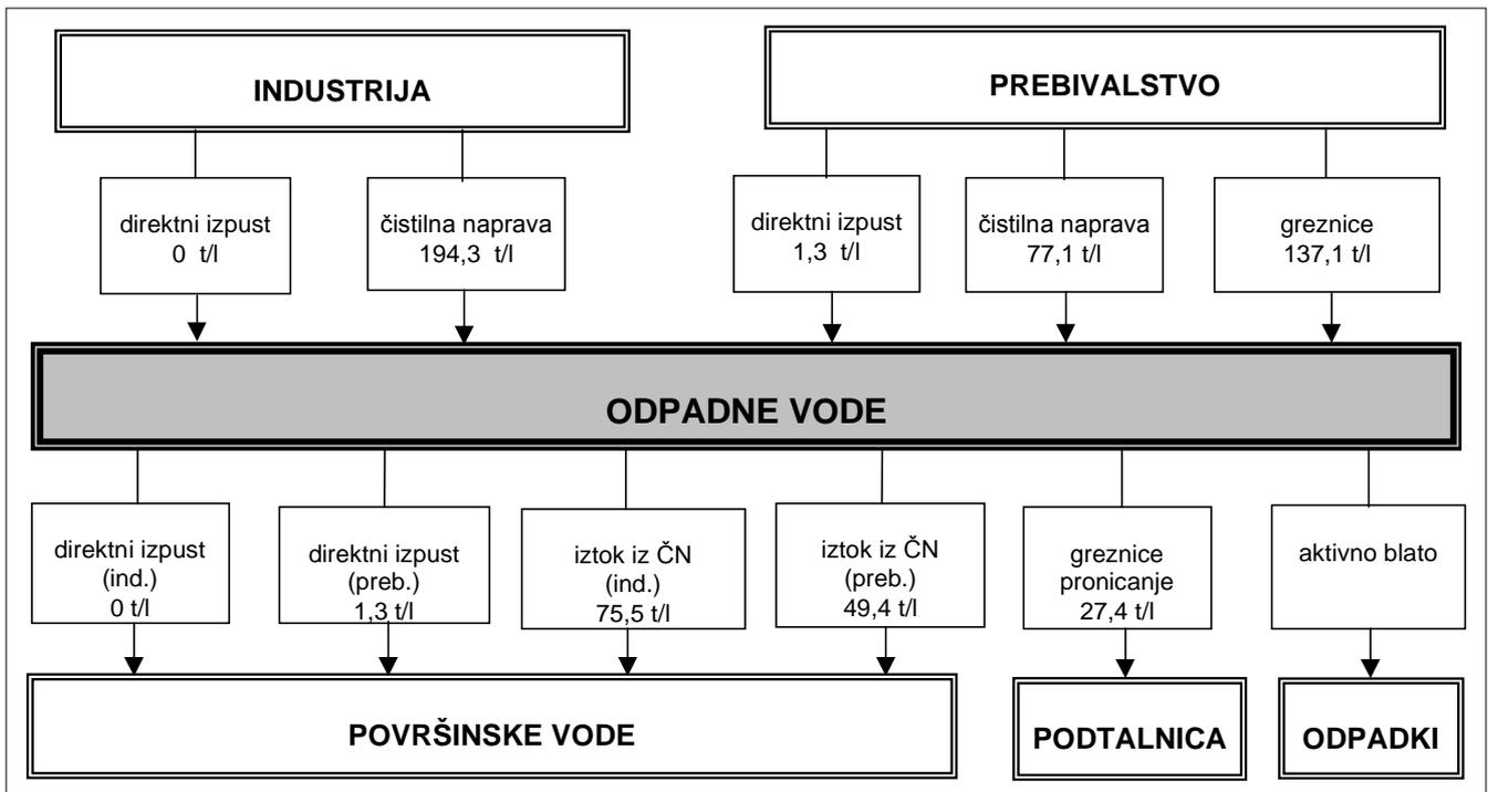
Figure 4: Process "waste water" for the lower Krka river basin
