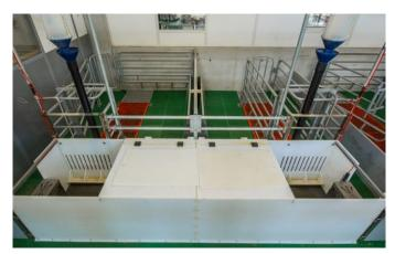
Figure 5: Pro Dromi-pen (left: crate open, right crate closed; © Pro-SAU)
