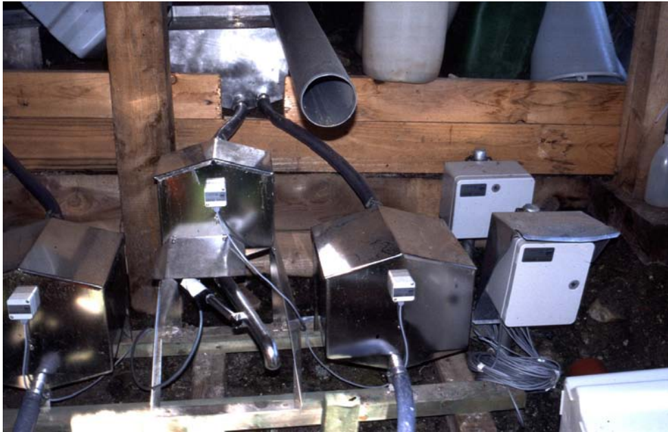
Photo 1. Tip pans of 0.5 and 2 litres of the erosion facility "Hochwurzten"
