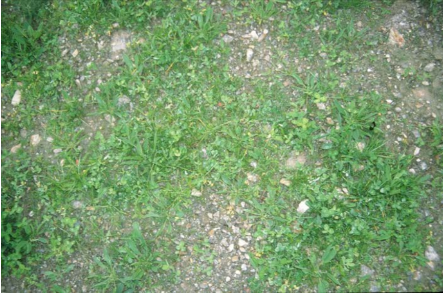
Photo 6. Vegetation cover on the plot with the technique Hydroseed a year after setup (2002), the fine-grained material was washed out
