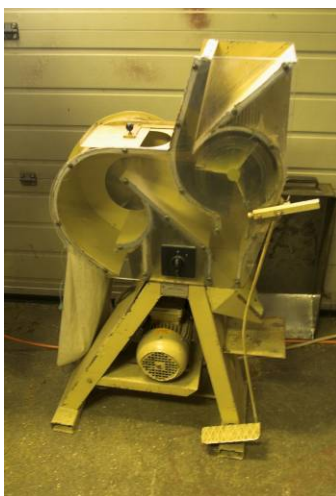
Figure 27: The Universal Threshing machine
