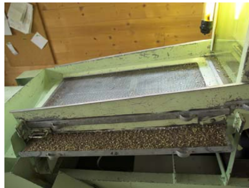
Figure 23: Detail of the two sieves on the Rober mini pectus
