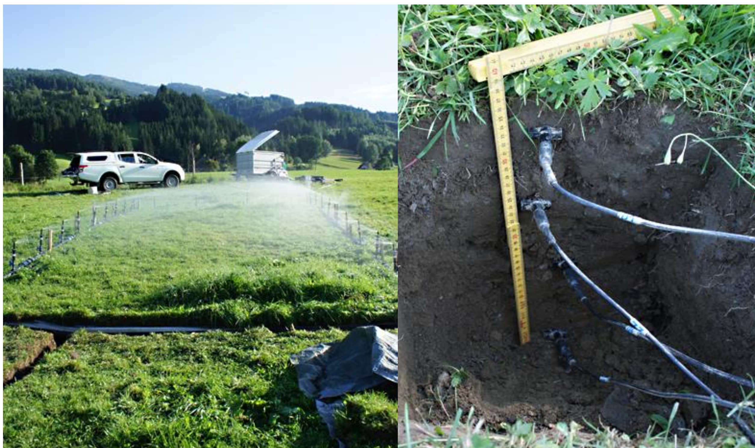
Figure 1: Measurement of surface runoff at five differently steep meadows and forest plots in the Upper Styrian Enns Valley. Source: https://www.bfw.gv.at/die-regenmacher-im-ennstal/
