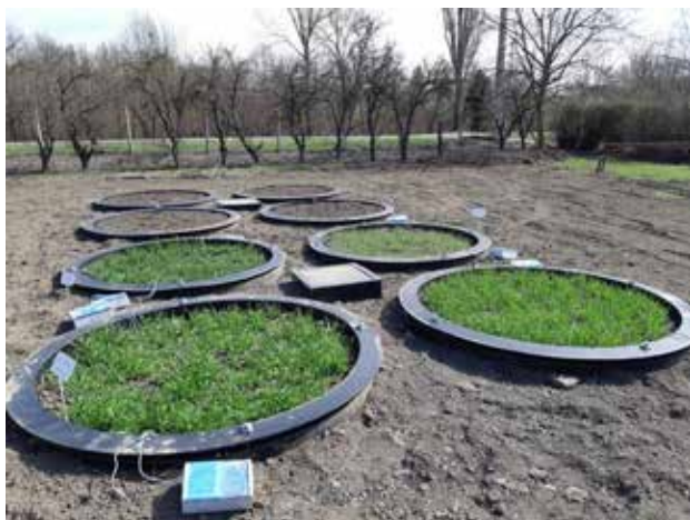
Figure 1: New weighted lysimeters (left) and the computer controlled precision irrigation system (Szarvas, Hungary).
