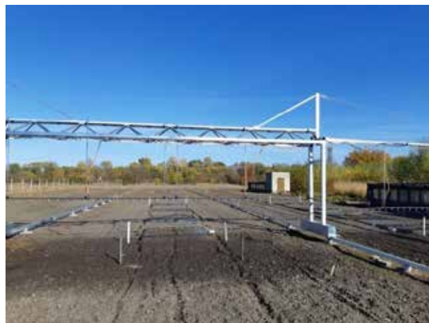
Figure 1: New weighted lysimeters (left) and the computer controlled precision irrigation system (Szarvas, Hungary).
