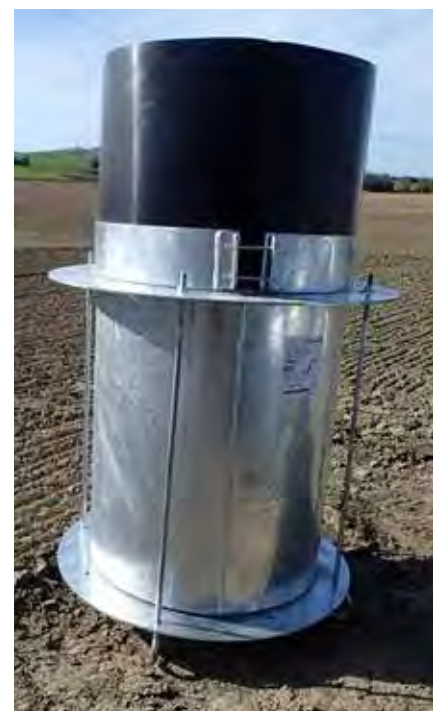
Figure 3: Arable lysimeter during design and after fabrication. The standard soil monolith lysimeter (500 mm diameter, 700 mm deep) was modified by the addition of a 400 mm polyethylene upper rim and clamp.
