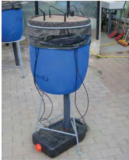
Figure 1: Modified wick lysimeter and drip irrigation system
