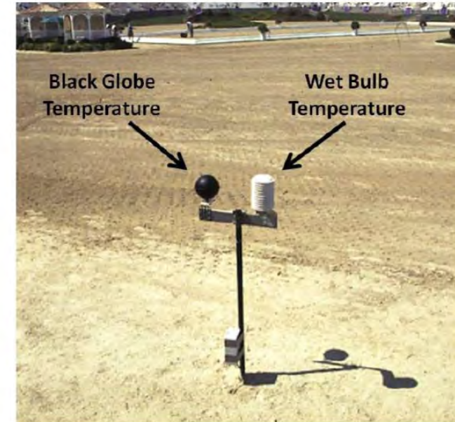
Figure 1. Equipment measuring WBGT index from black globe temperature (°C) and wet bulb temperature (°C) inside a shaded screen.
