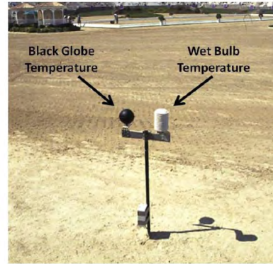
Figure 1. Equipment measuring WBGT index from black globe temperature (°C) and wet bulb temperature (°C) inside a shaded screen.
