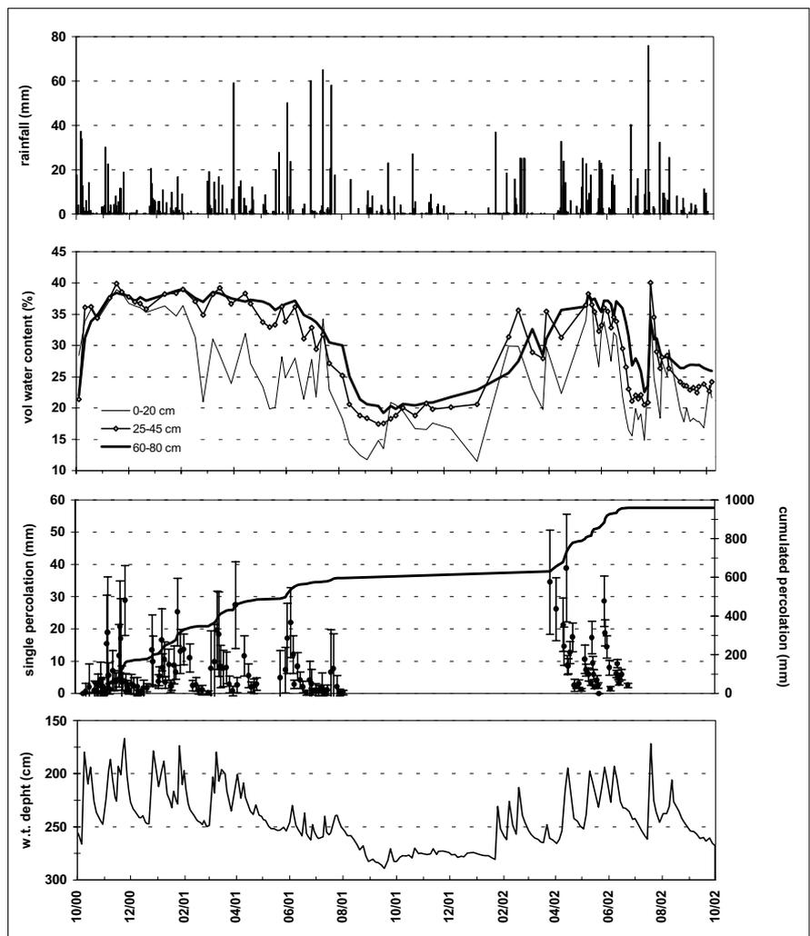
Figure 2: Rainfall, soil water content, percolation and water table depth during the monitoring period
