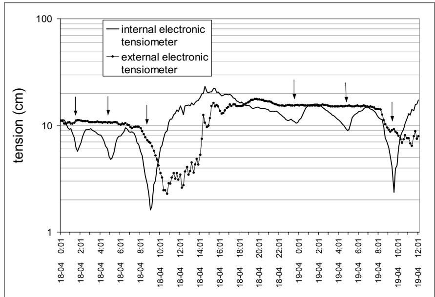
Figure 1: Example of automated activation of the vacuum pump according to soil potential measured above and beside the ceramic plates
