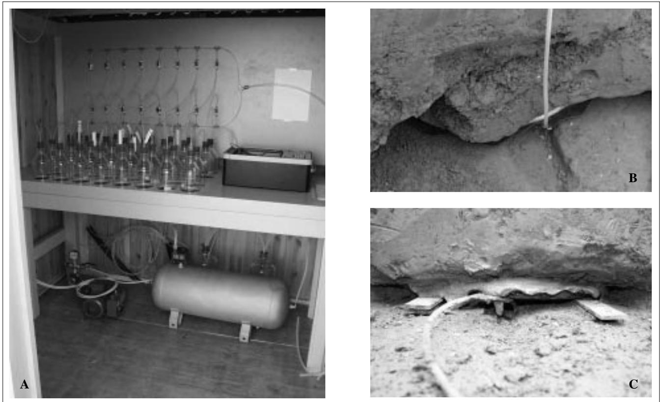
Figure 3 A): central components; B and C): installation of the ceramic plate (particulars)
