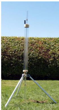
Abbildung 22: Guelph Permeameter (Soilmoisture Equipment Corporation 2008)
