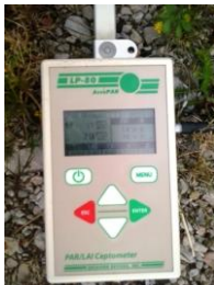
Abbildung 50: AccuPAR PAR/LAI ceptometer model LP-80 (Devices, D. 2008)
