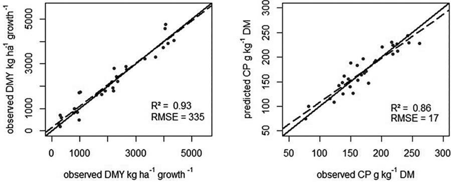
Figure 1. Observed vs predicted dry matter yield (DMY)  $\text{kg ha}^{-1}$  using rising plate meter (RPM) and leaf area index (LAI) from AccuPAR (left) and observed vs predicted crude protein (CP)  $\text{g kg}^{-1}$  dry matter (DM) using crop height and chlorophyll content (CC) from *Alopecurus pratensis* (random leaves) on the right side.
