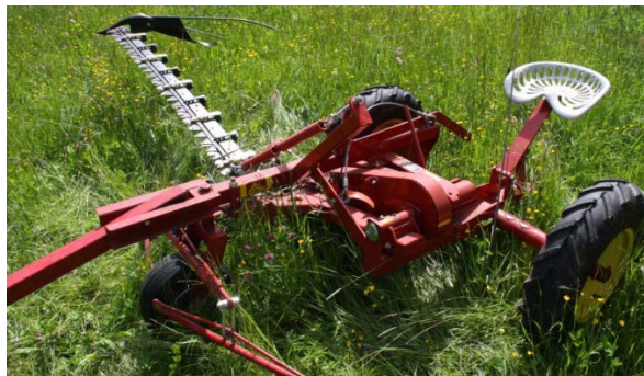
Figure 1: Mower with double knives: advanced technology, cutter bar is 2,2 m long, a three v-belts actuate the chain, very robust, does not plug up, best adapted for mowing meadows with horses, costs: about 6,800 € (Hohegger, Mayer, 2014)
