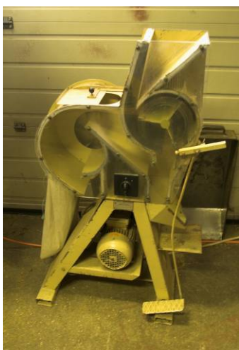
Figure 24: The Universal Threshing machine
