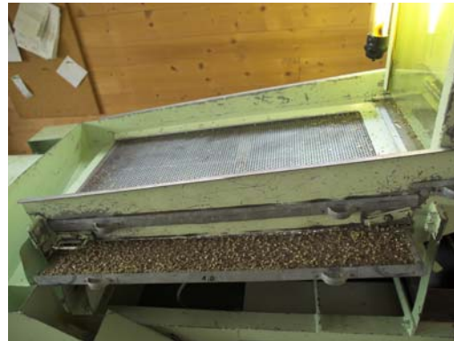
Figure 20: Detail of the two sieves on the Rober mini pectus
