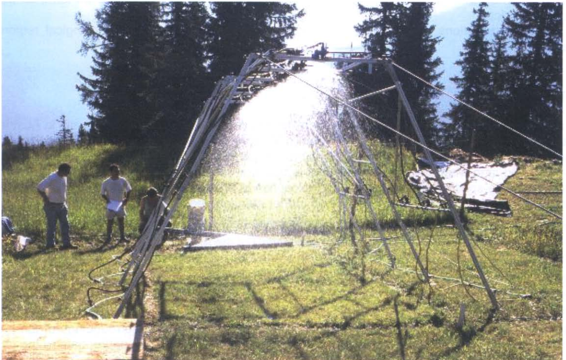
Figure 1. Rain simulations on slopes (experimental site Hochwurzen, 1.830 m) showed that a sufficient protection of the soil surface (e.g. by straw, hay) is necessary to avoid erosion the weeks after seeding.
