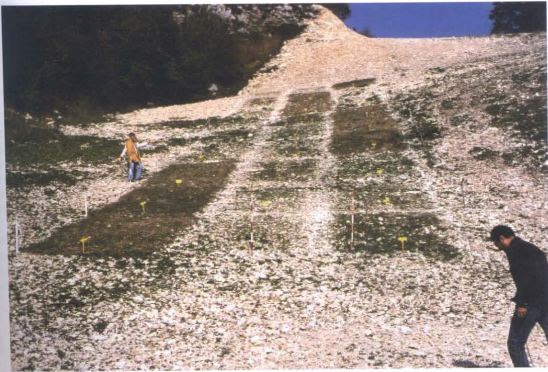
Figure 2. Under extreme site conditions, only a combination of high quality application technique with site specific seed mixtures or plant material leads to successful results (location Piancavallo, 1.435 m).
