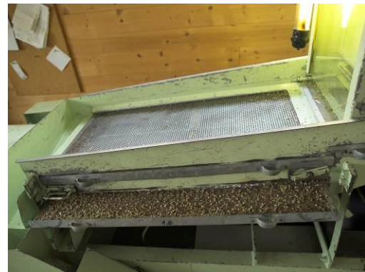
Figure 29: Detail of the two sieves on the Röber mini pectus
