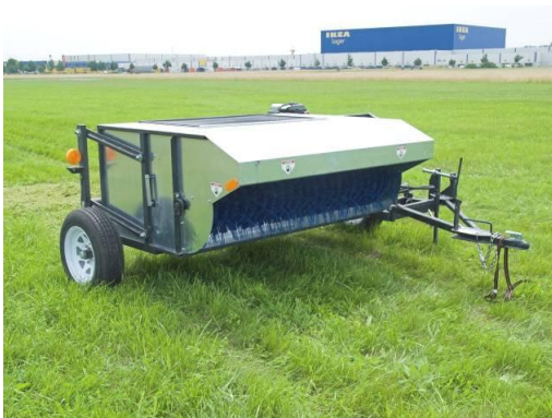
Figure 15: Pull-type seed stripper Model No. 610 imported from Canada
