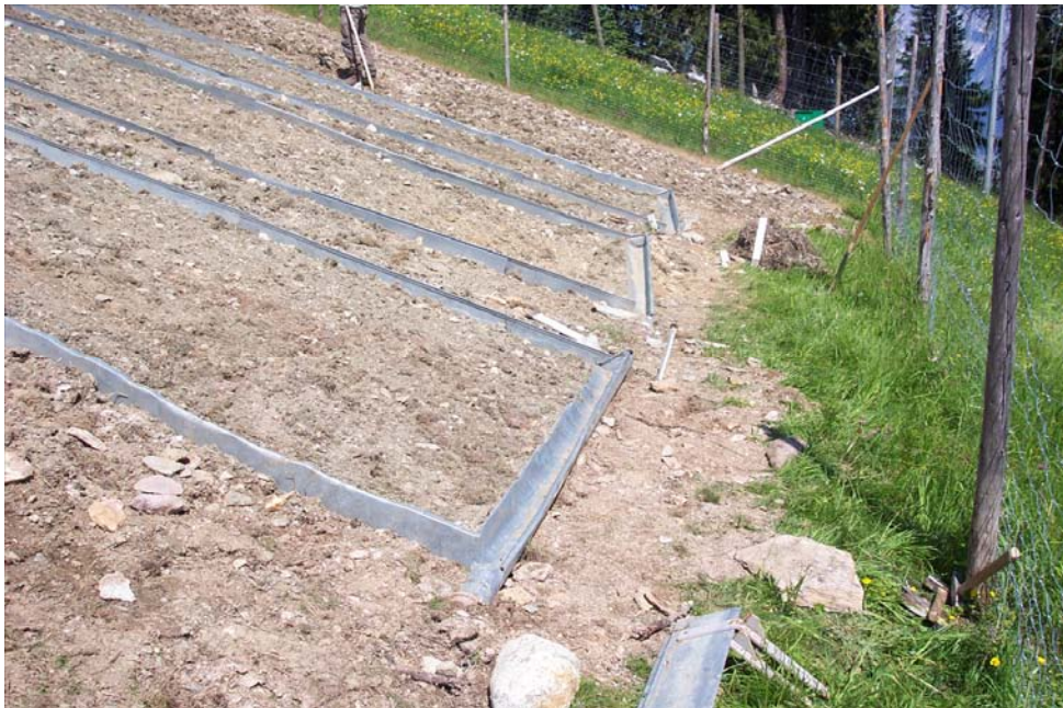
Photo 2. The collecting tube at the bottom of the plots
