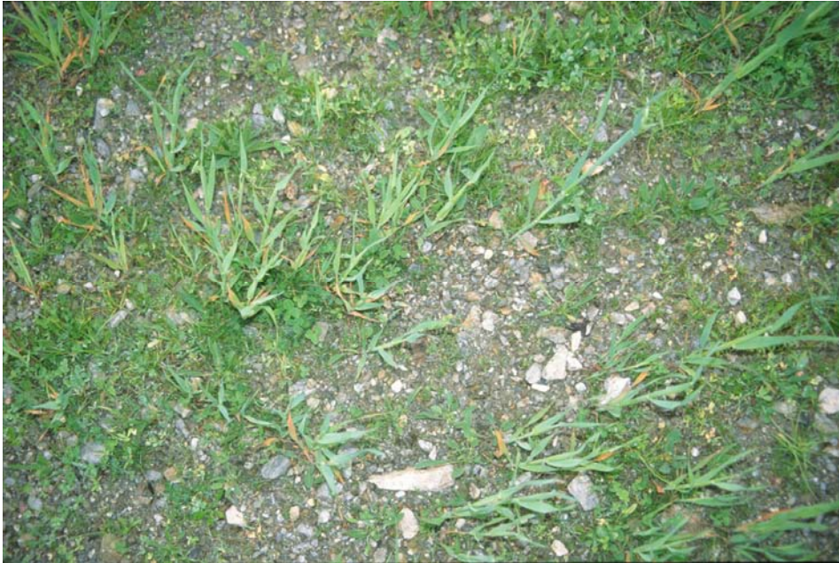
Photo 5. Vegetation cover on the plot with the technique hand sowing plus cover crop a year after setup (2002), the fine-grained material was washed out
