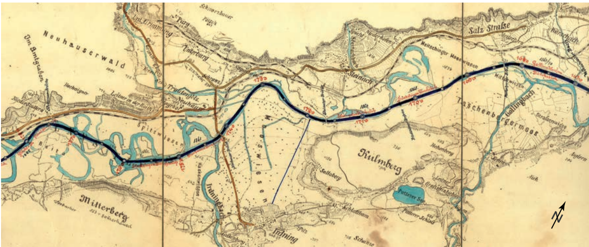
Figure 2 – Map of the regulation of the Enns, from Niederstuttern to Wörschach (Styrian Provincial Building Directorate, Graz 1859). Black line – regulated Enns; Blue – oxbow lakes, tributaries and lake; Brown line – roads; red numbers: river cuttings, see Figure 3.
