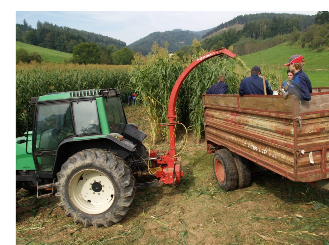
Fig. 2 Manual feed of sorghum plants in a single row chopper (Pöttinger) and ensiling of chopped material into plastic barrels on a forage wagon.
