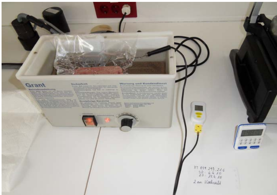
Figure 3. Meat sample cooking in the water bath
