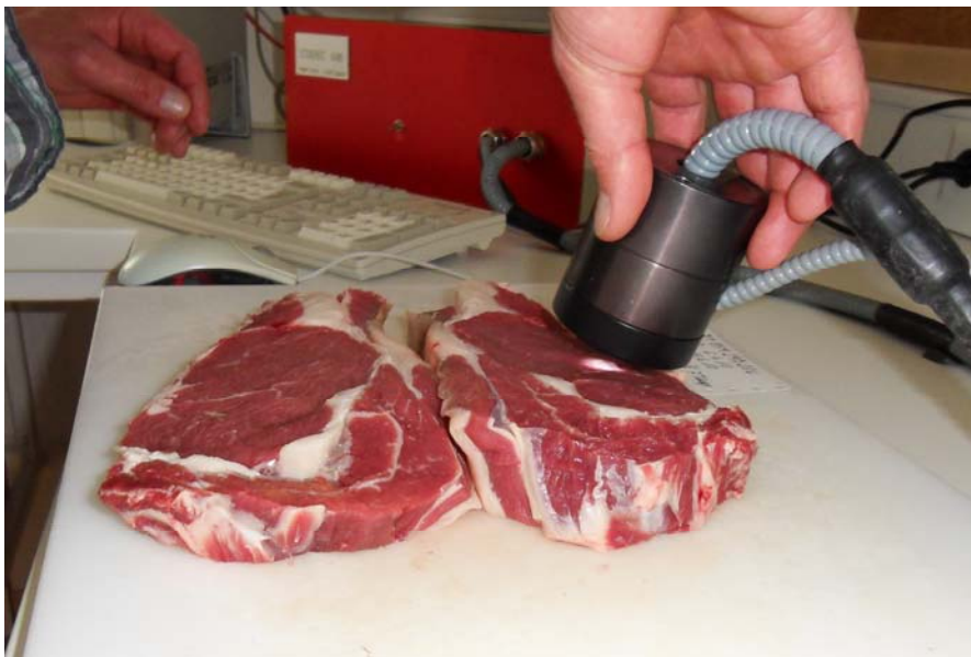
Figure 2. Meat and fat colour measurements with a spectrophotometer
