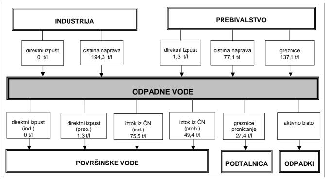
Figure 4: Process "waste water" for the lower Krka river basin
