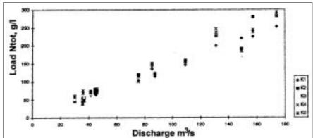
Figure 3: Nitrogen load versus discharge for river Krka (from DROLC, 1998)
